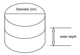
**FORMULA 1**: Volume (in litres) = 0.8 x water depth (cm) x diameter<sup>2</sup> (cm<sup>2</sup>)  $\div$  1000
